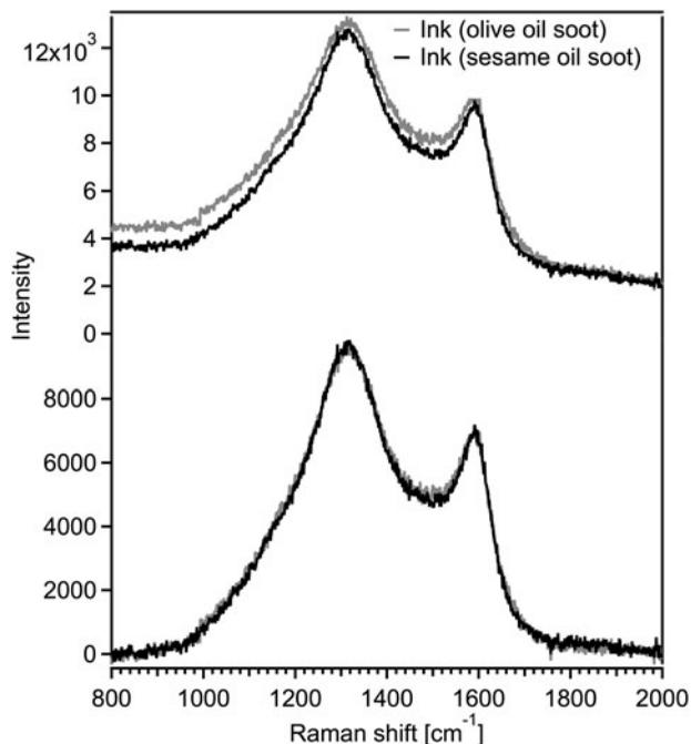
Figure 6. Comparison of the Raman spectra of inks based on the soot produced from sesame oil (black) and olive oil (grey). The spectra were collected with  $\times 20$  objective at the excitation line of 785 nm. Top: original spectra; bottom: after subtraction of the linear baseline
